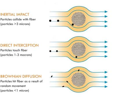
Particles larger than three microns are collected when their momentum prevents them from following gas streamlines around fibers. They leave the streamline, strike a fiber and are collected by the filter.
