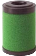
Our "C1" element is our 1 micron coalescer and is the equivalent of our old Grade 8 or Grade 10 elements. **Green in color**, this coalescer is normally used as a pre-filter to a C series grade filter to extend its life. Used to remove gross amounts of water and oil, or tenacious aerosols that are difficult to drain.
