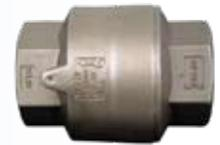
Process Lines 2" and larger use a wafer type check valve which has all stainless steel internals and a vulcanized sealing seat. The seat is located on the trailing edge of the process flow protecting it from the damaging desiccant dust.
