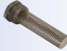
The Great Lakes Air desiccant support screens are fabricated from heavy gauge perforated stainless steel. The perforation pattern is designed to retain the desiccant bed while allowing small particles to pass, this prevents particle buildup and high pressure drops. Screens with tighter perforations or wire mesh covers run a high probability of damage from pressure drop. The screens are 100% welded construction, with no epoxy bonding.
