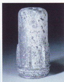
Rapid corrosion of untreated aluminum
