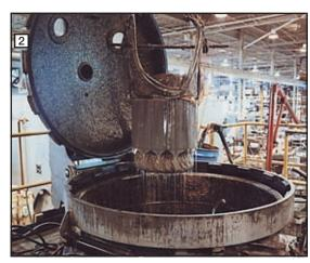
To withstand humid marine environments, Reliance Navy motors use standard U.S. Navy insulation systems meeting MIL-I-24092 specifications. For critical applications, a sealed insulation system is also available, which meets MIL-M-17060E requirements including 200 hours of submerged qualification testing and a 24-hour underwater stator winding production test.
