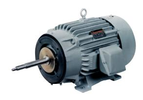
7.5-HP, 3600-RPM TEFC close-coupled pump motor designed for low structure-borne vibration, with a threaded Monel® shaft per MIL-P-17840.
