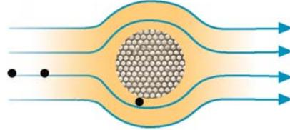
Particles between 1.0 and 3.0 microns tend to follow the gas streamlines as they flow relatively close to fibers. A 1.0 micron particle, for example, passing within 0.5 micron of a fiber will be collected by the fiber.
