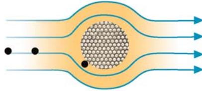
Particles larger than three microns are collected when their momentum prevents them from following gas streamlines around fibers. They leave the streamline, strike a fiber and are collected by the filter.
