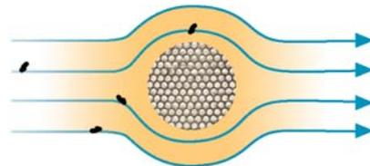
Extremely fine particles have random side-to-side movement caused by collisions with gas molecules. A 0.1 micron particle will have about ten times the Brownian movement or random motion of a 1.0 micron particle, greatly increasing the probability of collision with a fiber.
