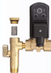
Great Lakes dryers utilize high quality diaphragm type solenoid valves as drains in addition to an isolation valve and strainer. Diaphragm valves isolate contaminants from the internal piston that would normally foul and restrict its movement causing failure. Diaphragm valves also have much larger orifices and flow paths that in conjunction with the strainer virtually eliminates the possibility of clogging a condensate drain valve.
