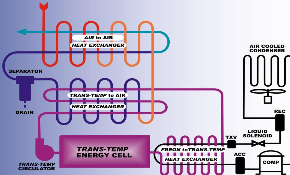
The **Trans-Temp Energy Cell™** integrates a proprietary blend of non-hazardous, completely biodegradable fluids that attains an ideal balance of thermal storage and thermal conductivity. The energy cell is encased in a heavy duty non ferrous vessel that is insulated to maintain energy efficiency.
