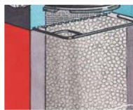
Snow Storm filled to prevent fluidisation and channelling
